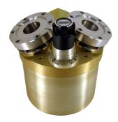
The Resonance Ltd. vacuum monochromator and spectrometer uses standard connections to allow simple integration into most systems. The f/2.2 grating is a type 4 for minimal aberrations. It is designed to allow easy interchangeability between being a monochromator and a CCD-based spectrometer. It's supplied with LabView-based codes and drivers for integration into user software.
