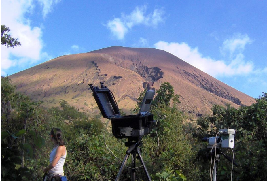
Fig. 4. A custom COSPEC at MASAYA Volcano in 2003 with PACA on separate tripod
