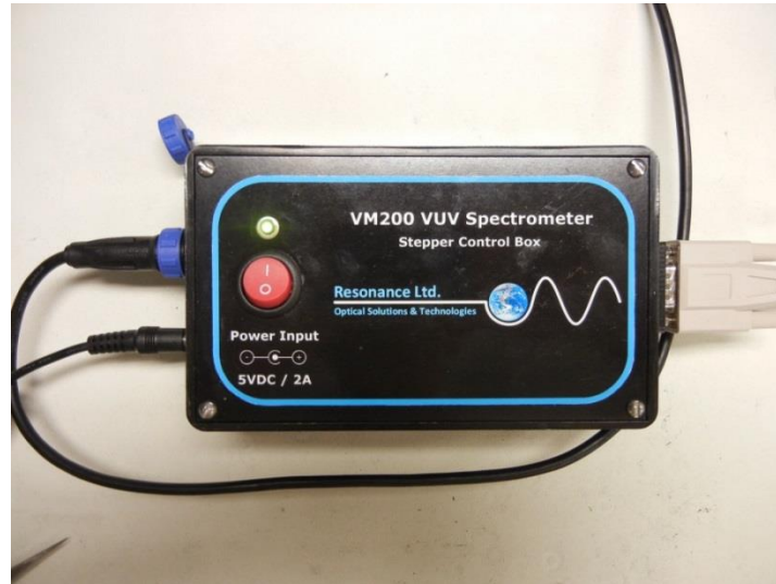
Figure 2: Motor Drive Controller Box
