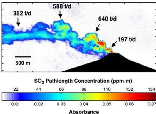
The concentration of SO<sub>2</sub> in the plume is designated by a colour gradient relating the arbitrary false colours to a numerical ppm-m concentration value. Figure 3 was generated after collected data was post-processed using 3<sup>rd</sup> party tools and therefore does not display the SO<sub>2</sub> concentrations in real-time.
