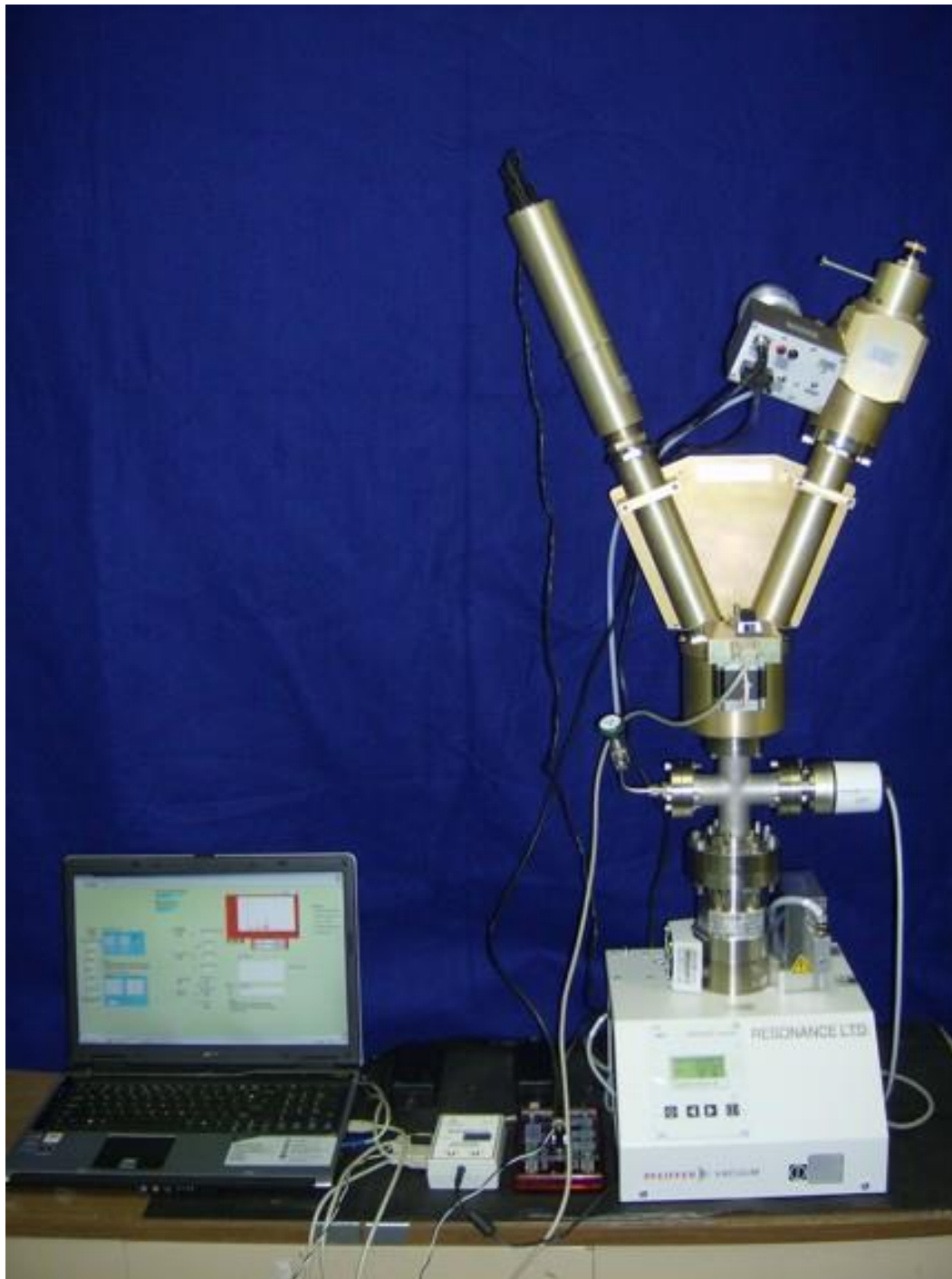
Figure 2: Tunable light source for TR-SES (note PMT on left top is placed inside sample chamber shown below)
