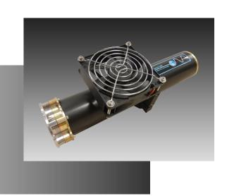
This Krypton filled RF powered lamp system is a reliable and maintenance free high intensity source of deep VUV emissions at **116.5 and 123.6 NM**. This source mounts to a 2.75 inch CF flange for convenient connection to a HV system. VUV fluxes greater than 3 milliwatts are delivered through the output window for use in vacuum applications such as photoluminescence, photoionization, photoliography and mass spectroscopy.
