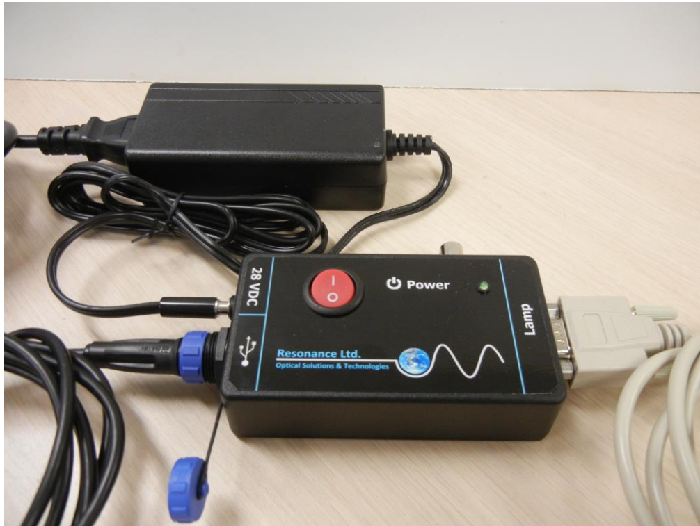
Above: The power/data Break-out box, with 28 V input, RS-232 telemetry, and Lamp connector.
