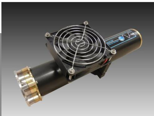
The Hydrogen Light sources come standard with everything needed to produce VUV radiation in the 110 to 200 nm region. A heater on the light source bulb generates H<sub>2</sub> or D<sub>2</sub> in the light source. This allows the user to operate the light source at low H<sub>2</sub> levels for an “optically thin” Lyman-Alpha line or a multiple-lined H<sub>2</sub> spectrum in the 110 to 165 nm region and a continuum between 165 and 375 nm.
