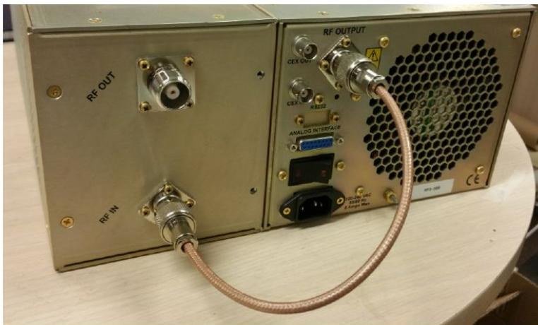
5. Connect the RF tuning box's RF output to the lamp's RF Input.
