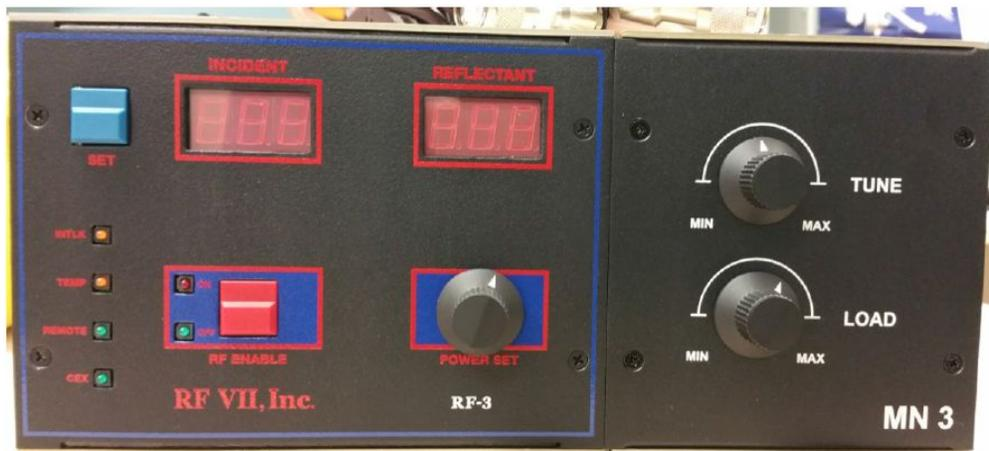
11. As long as the green "Fan OK" LED is lit, RF power can be enabled since its interlock should be satisfied. Press the "RF Enable" button to activate RF output. Adjust the amplitude (power) of the RF by turning the "Power Set" knob. We recommend using 25 Watts of RF power as an initial setting.
