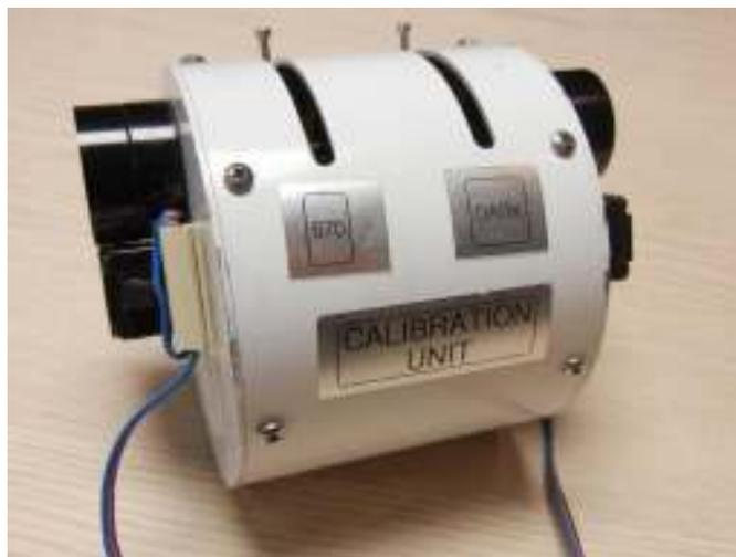
Fig. 7: The automatic gas cell changer add-on for the PACA.
