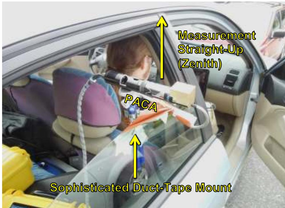
Fig. 14: The Expedition setup for Mode 1: Transverse (Vehicular).
