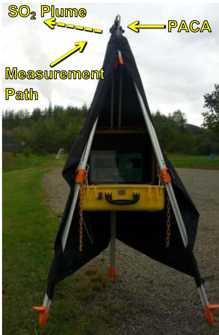
Fig. 15: The Expedition operating in Mode 2: Stationary Pointing at an SO<sub>2</sub>-producing stack in Sudbury, Ontario, Canada – while it's raining!
