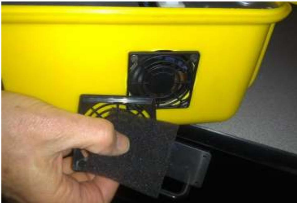
**Fig. 29: Removing the fan guard to reveal the filter.**
