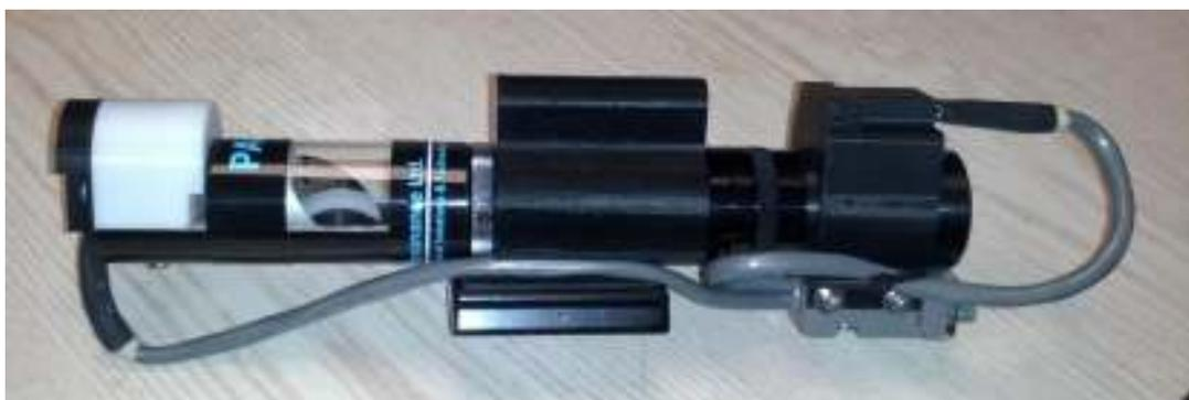
**Fig. 1: The PACA (Pointing and Calibration Assembly) as a detachable module.**
