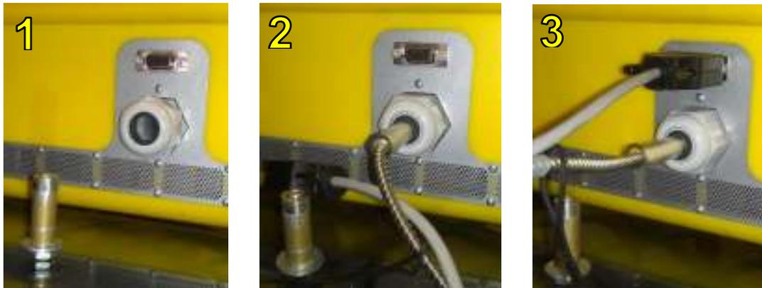
**Fig. 21: Connecting the fibre-optic to the main case.**
