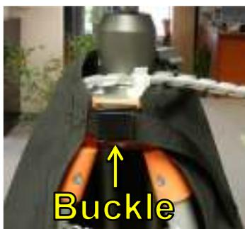
**Fig. 23: The installed Weather Shroud strapped around the tripod.**
