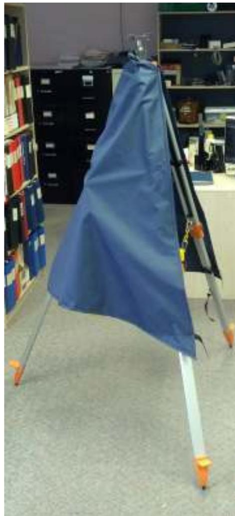
Fig. 12: The Expedition's tripod wrapped in the Weather Shroud.
